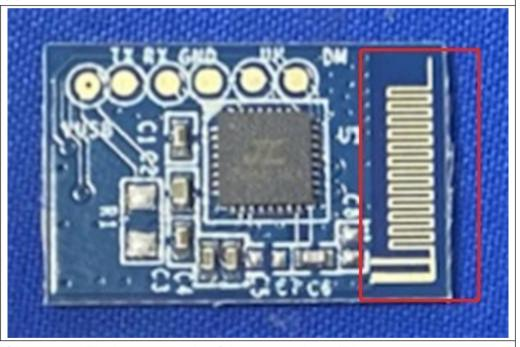
The antenna is PCB antenna. The best case gain of the antenna is -5 dBi.
