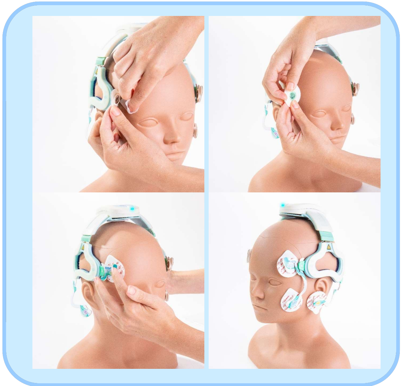
Figure 7-8: Electrode Pad Installation
