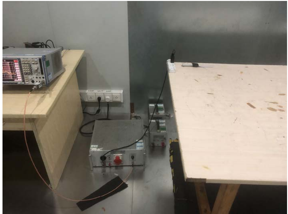
Conducted Emission Test Setup
