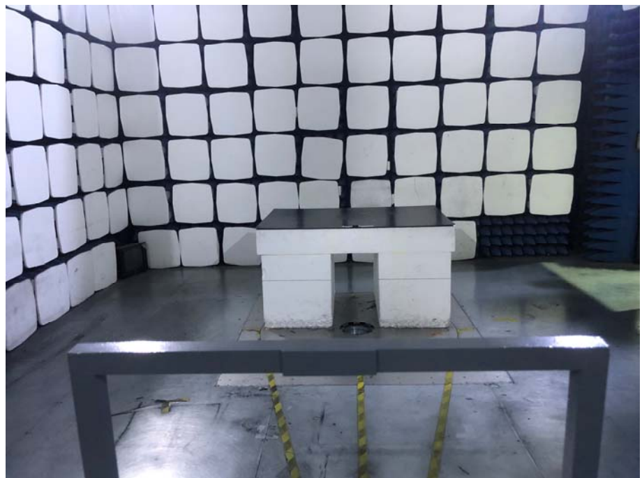
Radiation Emission Test Setup (Below 30MHz)
