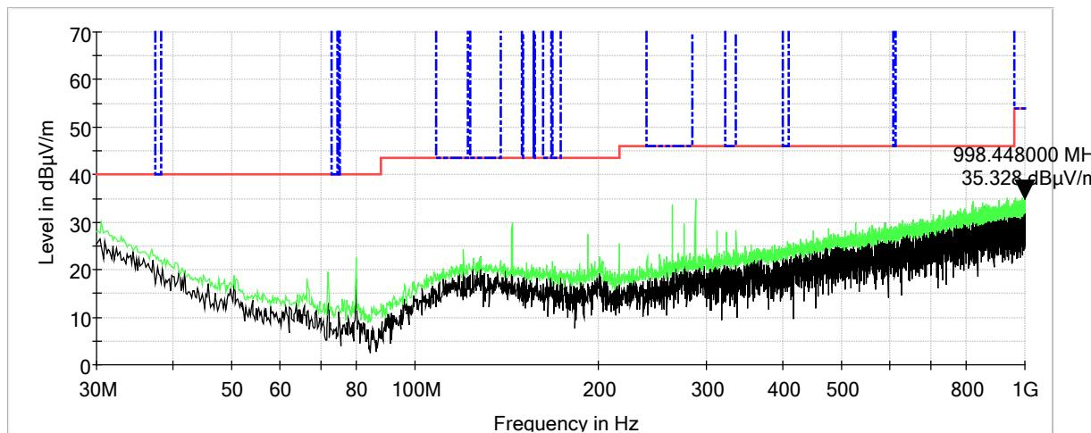
**Note: No signals between 1-26 GHz, other than the fundamental frequency, are within 20dB of the limit.**
