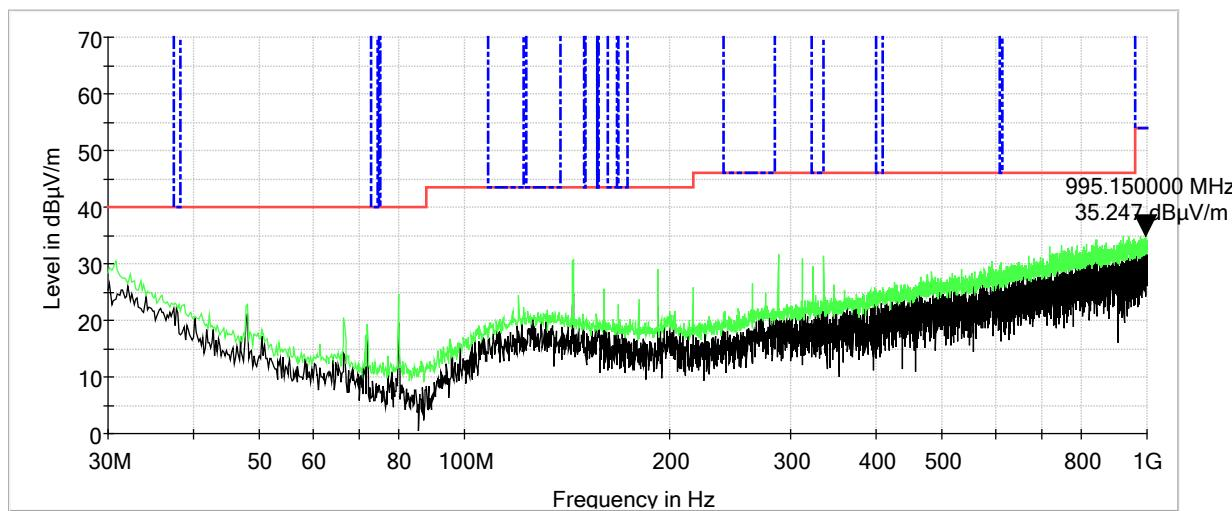
**Mid Channel, 30 MHz to 1000 MHz, Vertical**
