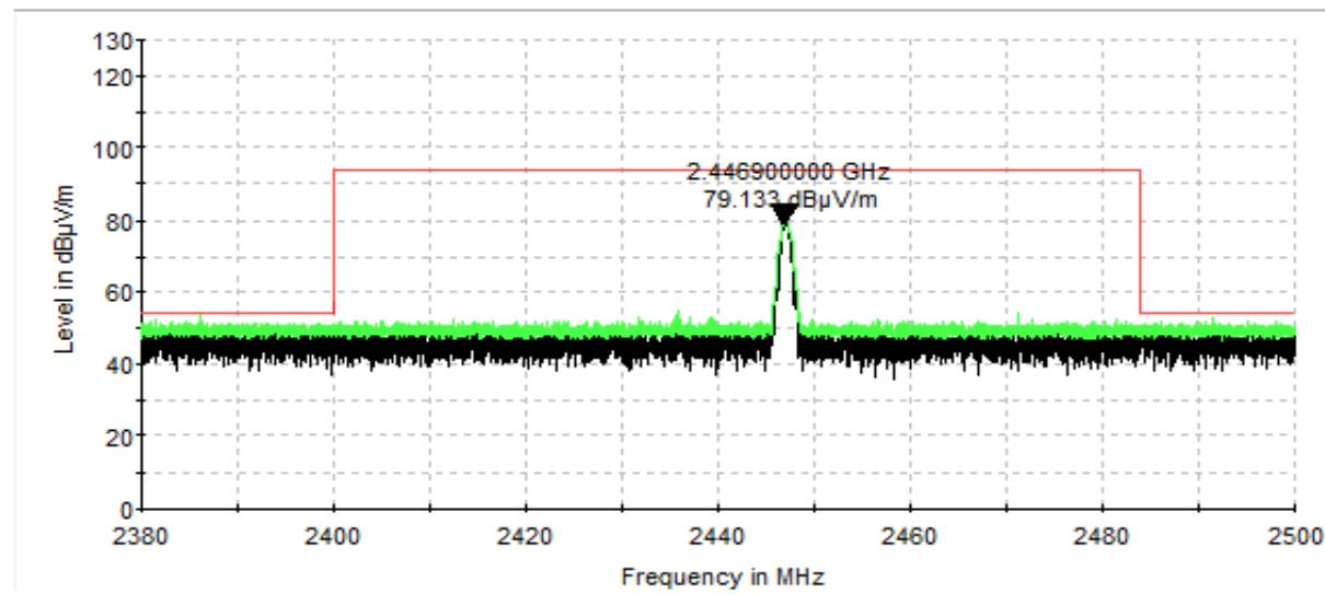
**Band Edge and Field Strength of the Fundamentals**
