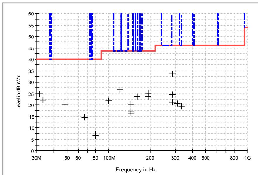
**Low Channel, 30 MHz to 1000 MHz, Vertical**
