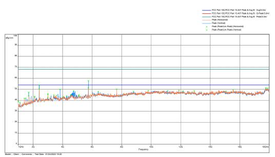
Note: 2412MHz peak is fundamental frequency of the 2.4GHz radio.
