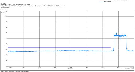
Frequency Amplitude Limit Margin Pass / Fail? Detector (MHz) (dBuV/m) (dBuV/m) (dB) 4823.7 Pass Average 49.6 54.0 -4.4 5150.0 Pass Average 47.81 54 -6.19
