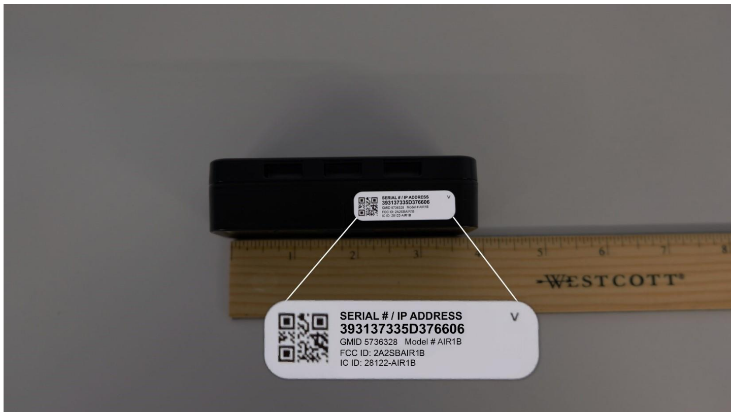
Figure 1: Final FCC & IC ID 2A2SBAIR1B Label Placement and Rendering for ActiveSense AIR1B Sensor
