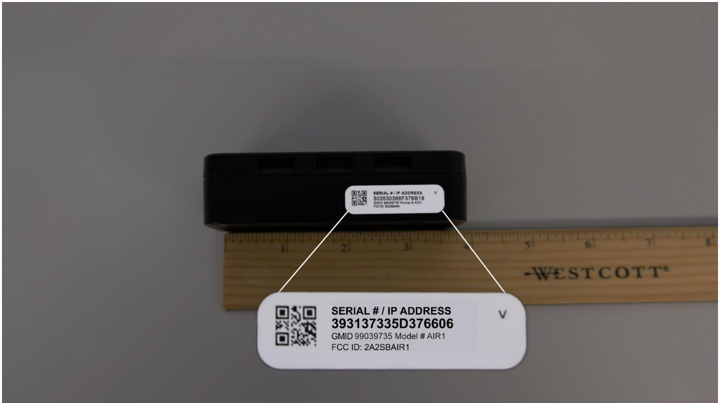
Figure 1: Final FCC ID 2A2SBAIR1 Label Placement and Rendering for ActiveSense AIR1 Sensor
