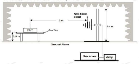
(3) Radiated Emission Test-Up Frequency Above 1GHz
