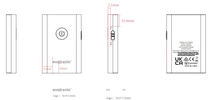
The Label's material is silk-screen, it cannot be easily erased. The MIC Logo height is 3mm\*3mm.
