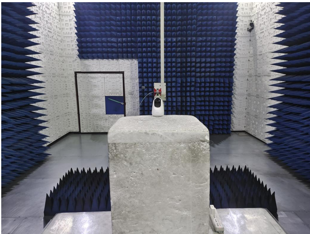
RADIATED EMISSION TEST SETUP ABOVE 1GHz
