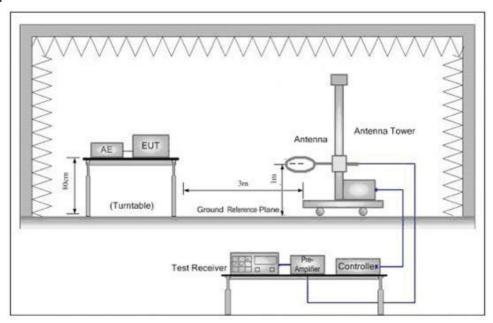
The test setup for emission measurement from 30 MHz to 1 GHz.
