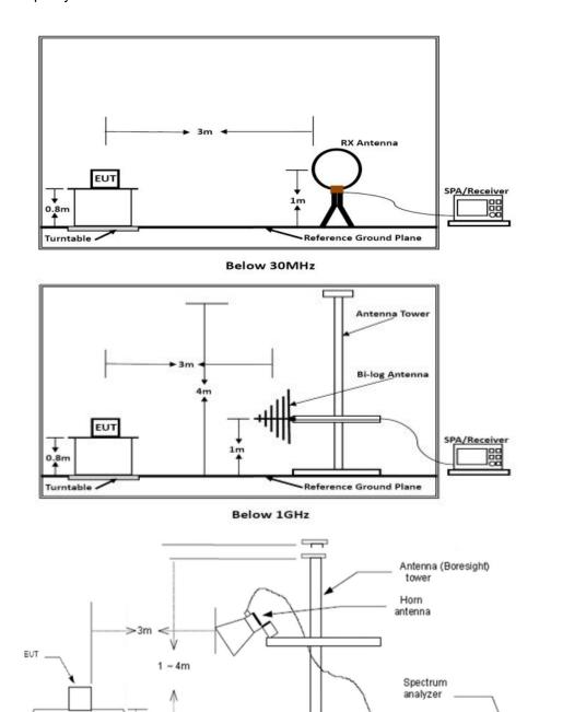
Above 18 GHz shall be extrapolated to the specified distance using an extrapolation factor of 20 dB/decade form 3m to 1m.
