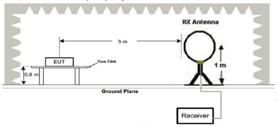
2. Radiated Emission Test-Up Frequency 30MHz~1GHz
