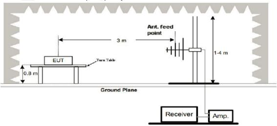
3. Radiated Emission Test-Up Frequency Above 1GHz
