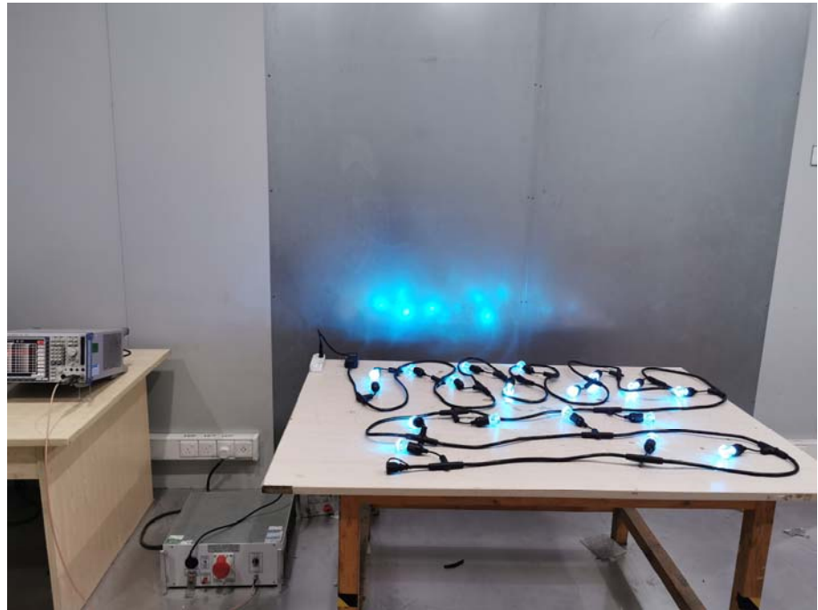
Conducted Emission Test Setup
