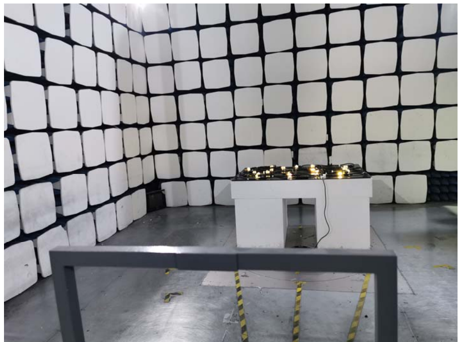
Radiation Emission Test Setup (Below 30MHz)
