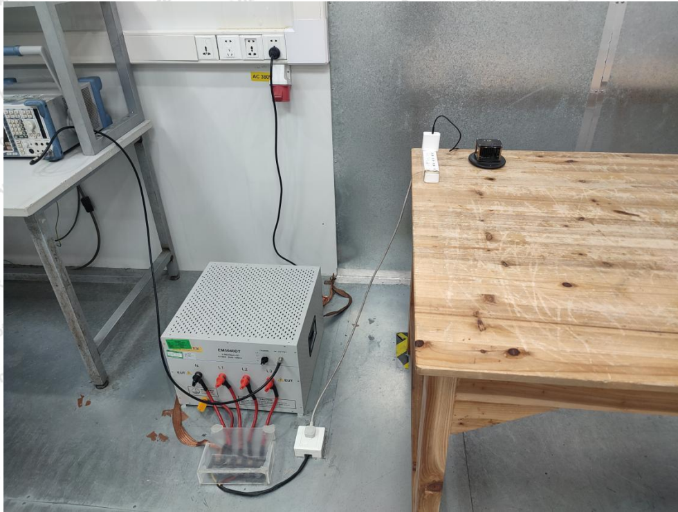
Photo of Conducted Emission Measurement
