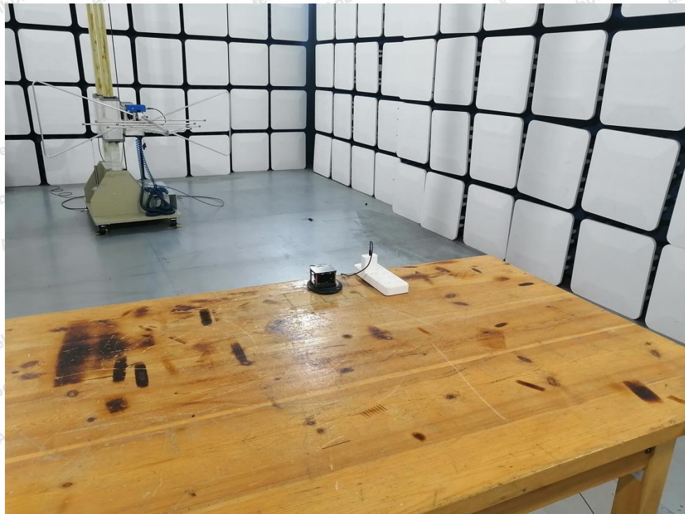
Photo of Radiation Emission Test
