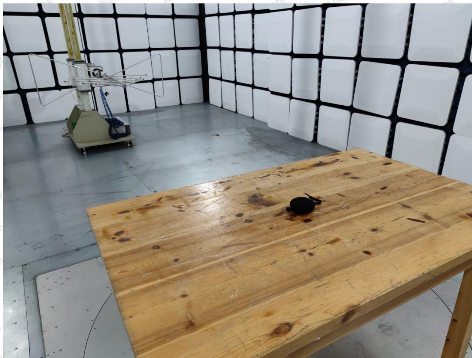
Photo of Radiation Emission Test
