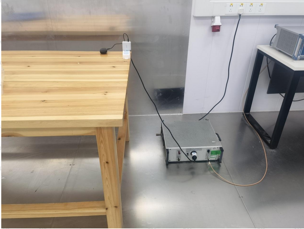
Photo of Conducted Emission Test
