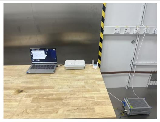
Radiated Emissions and Band Edge Measurement
