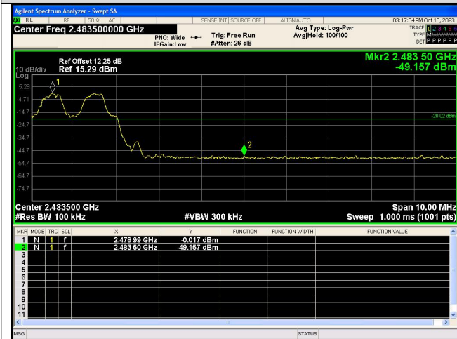
Out Of Band Emission(Right) GFSK_DH5_Channel Hopping
