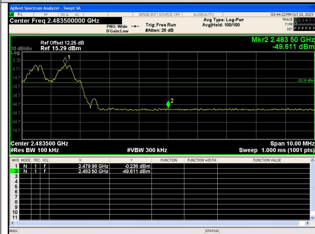
Out Of Band Emission(Right) GFSK_DH5_Channel Hopping
