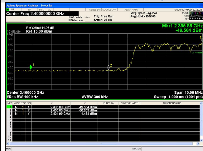
Out Of Band Emission(Left) 8DPSK_3-DH5_Channel Hopping
