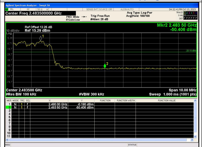
Out Of Band Emission(Right) 8DPSK_3-DH5_Channel Hopping
