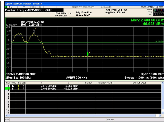
Out Of Band Emission(Right) GFSK_DH5_Channel Hopping
