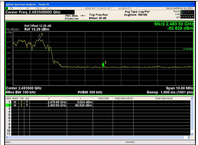
Out Of Band Emission(Right) \pi/4 DQPSK_2-DH5_Channel Hopping
