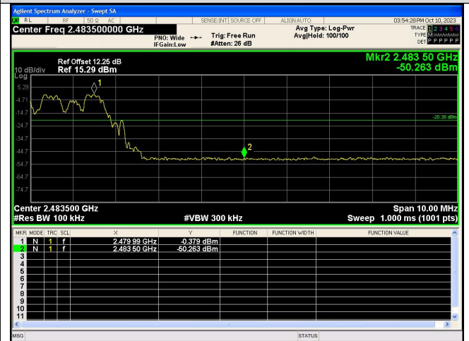
Out Of Band Emission(Right) \pi/4 DQPSK_2-DH5_Channel Hopping
