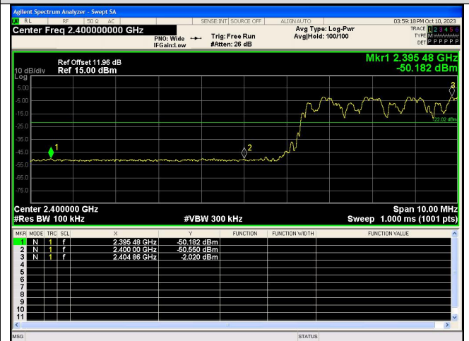
Out Of Band Emission(Left) \pi/4 DQPSK_2-DH5_Channel Hopping
