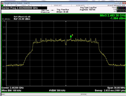
In-Band Reference Level IEEE 802.11g_Channel 11_20MHz_Antenna 0
