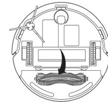
3. Use the matching cleaning brush to sweep away the dust in the main brush and the main brush cavity, and then Clean up the tangles on the main brush.
