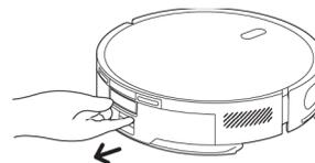
2. Press and hold the dust bin switch to open the dust bin and dump the garbage.
