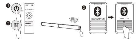
Short press the "BT" button on the remote control to enter Bluetooth mode. When entering the pairing mode, bb starts to flash, and the voice prompts "Paring", and pairing is successful, the voice prompt "Connected"
