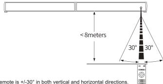
The working range of the remote is +/-30° in both vertical and horizontal directions.
