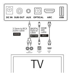
After connecting the line, use the buttons on the remote control or on the sound bar to change the input mode.
