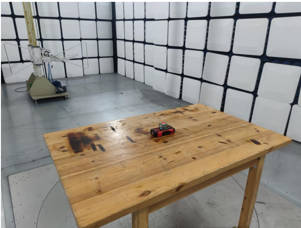
Photo of Radiation Emission Test
