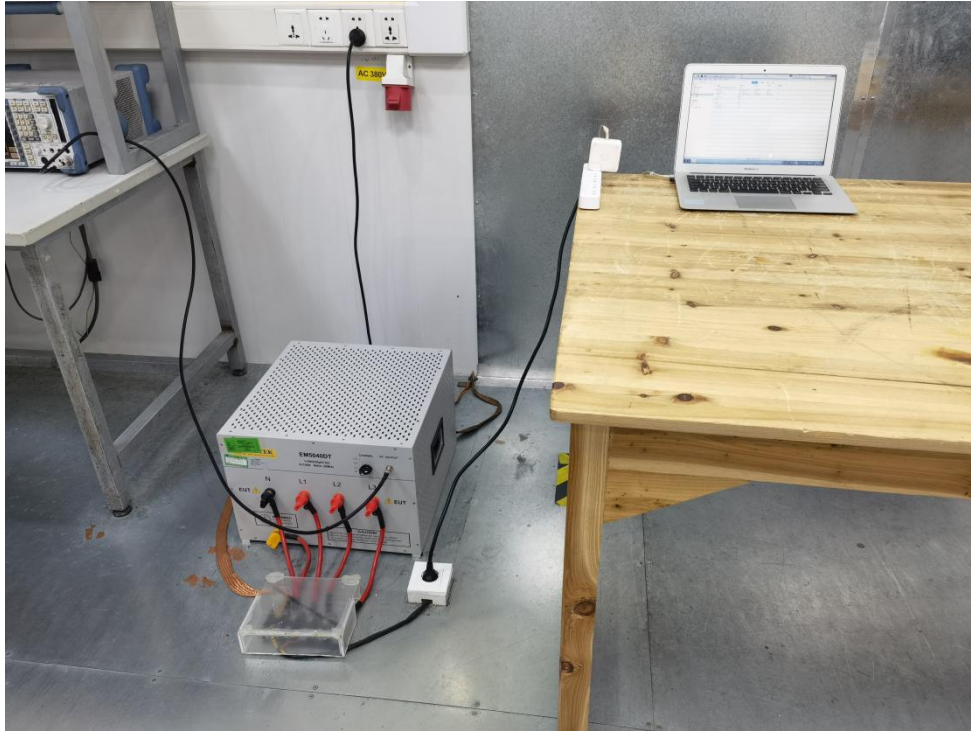
Photo of Conducted Emission Measurement
