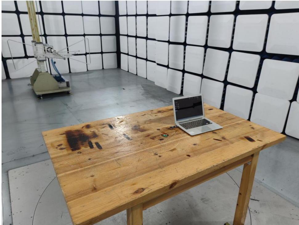
Photo of Radiation Emission Test
