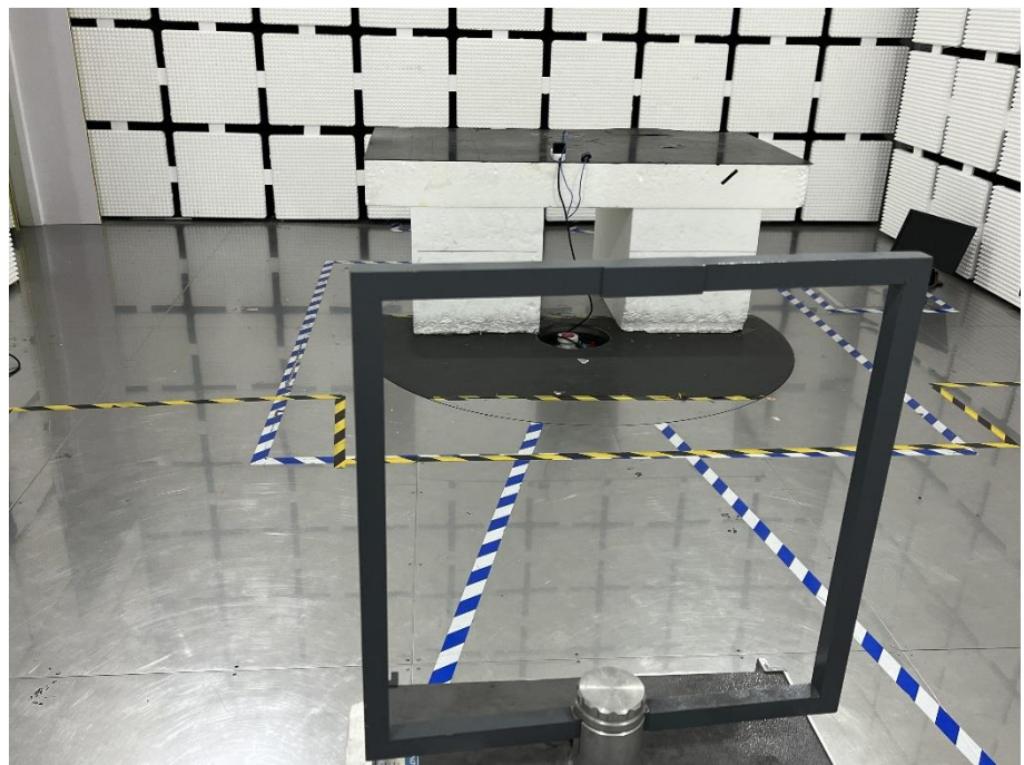
Radiation Emission Test Setup (Below 30MHz)
