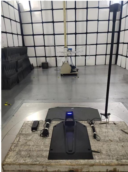
Photo of Radiation Emission Test
