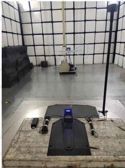
Photo of Radiation Emission Test
