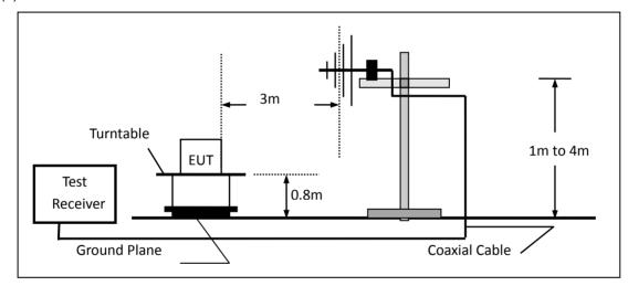
(c) For radiated emissions above 1000MHz
