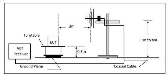
(c) For radiated emissions above 1000MHz
