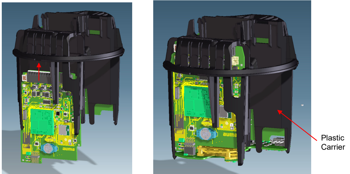
Figure 1: Integration of the Module Z139.910 in a plastic carrier
