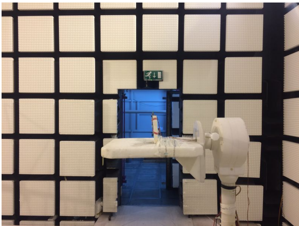
Photo 4: RSE setup < 30 MHz and > 1GHz
