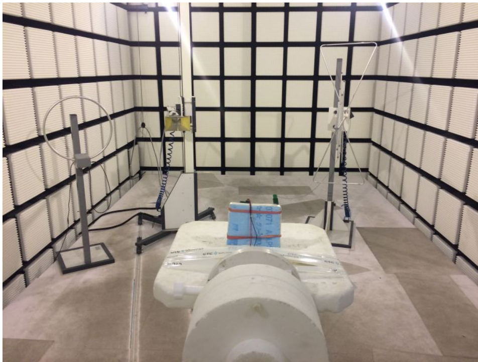
Photo 5: RSE setup < 30 MHz and > 1GHz
