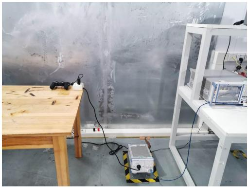
Test Setup Photo(s) of Conducted Emissions Measurement
