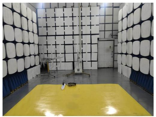
Test Setup Photo(s) of Radiated Emissions Measurement
