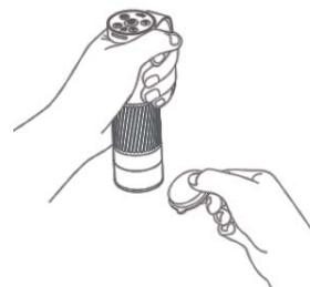
❖ Align the lens of the microscope at the object to be observed.
