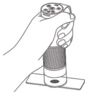
❖ Rotate the focus wheel with the other hand and observe the display of the phone. At this time, you can adjust the focus wheel to the best viewing ratio.
