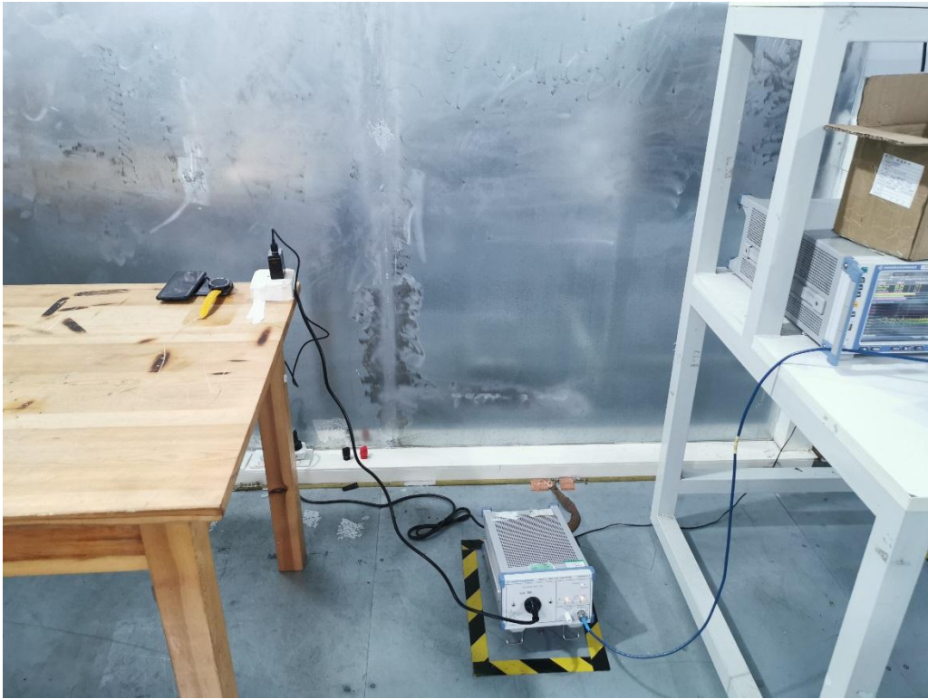
Conducted Emission-AC adapter charge mode
