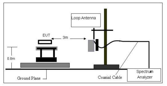
(B) Radiated Emission Test-Up Frequency 30MHz~1GHz
