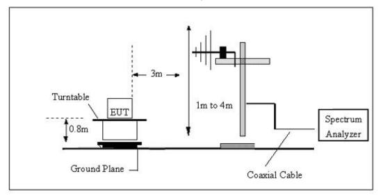
(C) Radiated Emission Test-Up Frequency Above 1GHz
