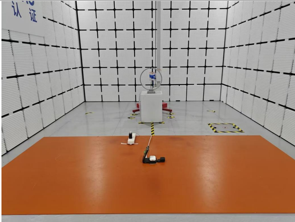
Radiated Emission Above 30MHz
