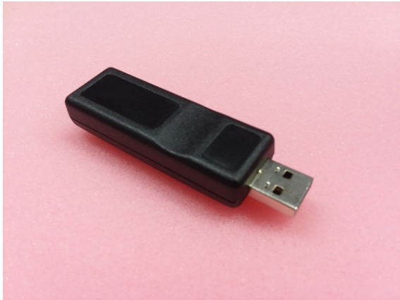
Figure 1. Photo. Coordinator dongle.
