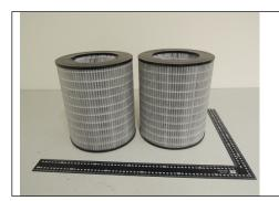
Photo of internal filter, the different filters are made up of different materials and different filters can filter different gases
