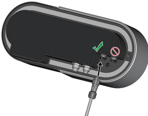
Fig. 12: Connecting the power cable
