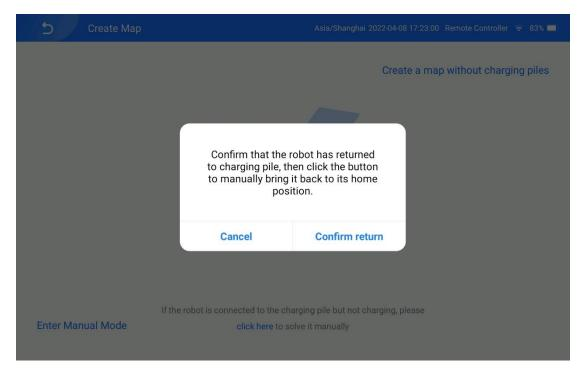
If the robot is not in the position of the charging pile, the following screen is displayed. Tap **Manual Mode** and remotely move the robot to the position of the charging pile for charging. Tap **OK** when the message above is displayed.
