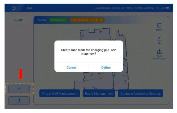
[3] Move the robot and connect it to the charging pile as prompted.
