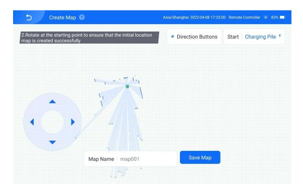
[6] Use the direction buttons on the left part of the screen to make the robot travel around the area to be disinfected and then return to the charging pile. Then, name the map and tap **Save Map**.
