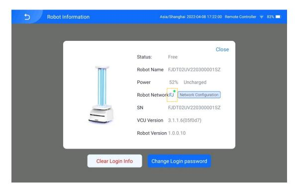
Enter the password of a local Wi-Fi to connect the tablet remote controller to the local Wi-Fi.
