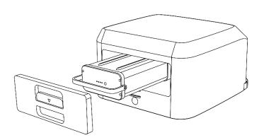
2. Connect the charging plug of the adapter into the battery charging port.
