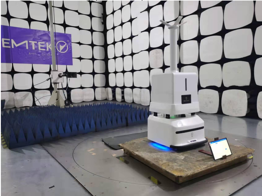
Spurious Emission Test Setup (Above 1GHz)
