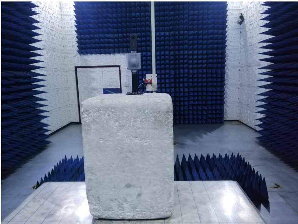
RADIATED EMISSION TEST SETUP ABOVE 1GHz
