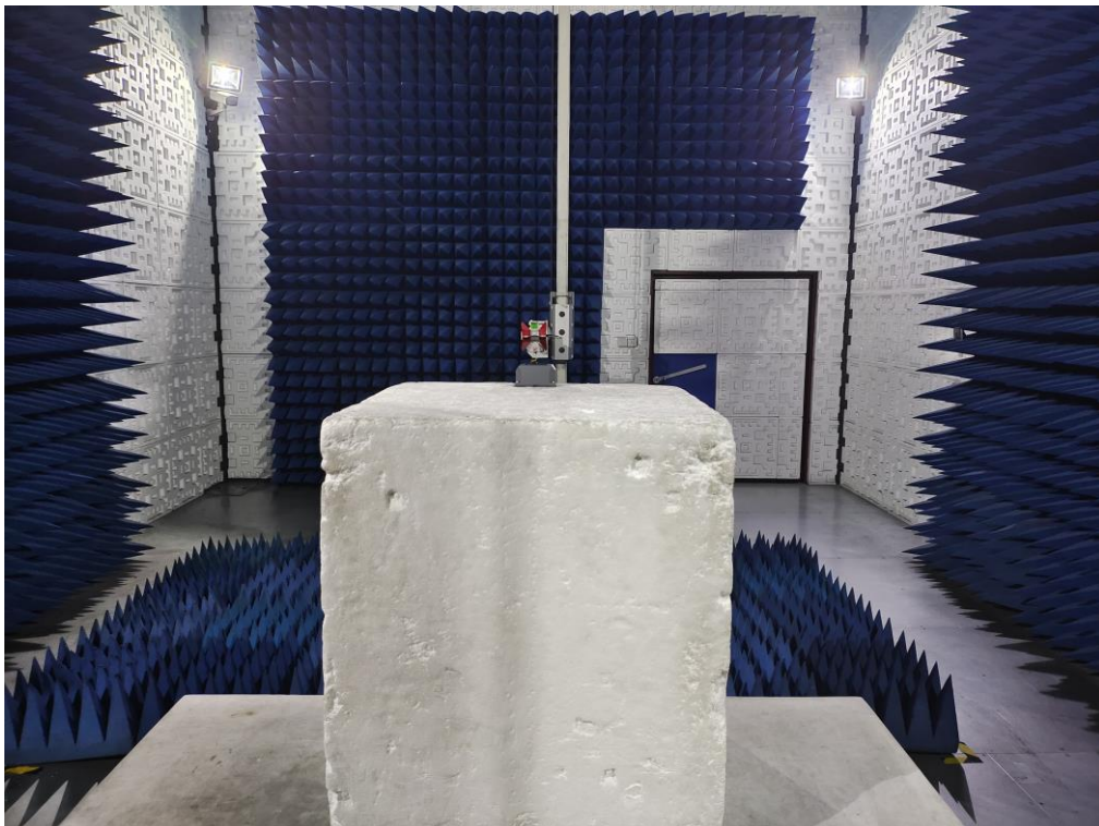
RADIATED EMISSION TEST SETUP ABOVE 1GHz
