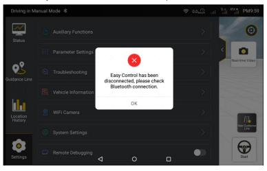
Figure 9 Bluetooth disconnected
