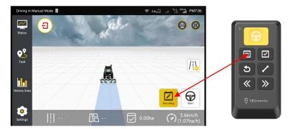
Figure 11 Turn on/off area metering
