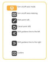
Figure 1 Functions of the FJD Easy Control
