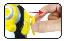
Have an adult open the battery door on the back of RoboEar with a Phillips head screwdriver (not included) and insert 3 "AAA" batteries (not included). Then replace the battery door and securely fasten with screw.
