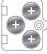
Install 3 button cell batteries into backpack as shown.
