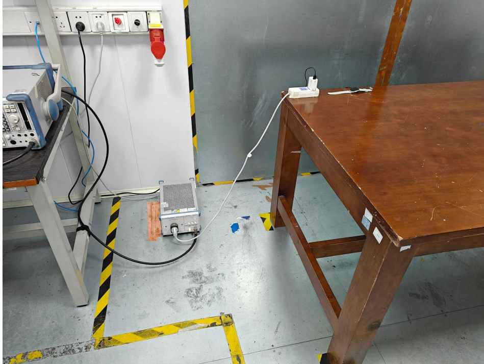
Conducted emissions at AC power line (150kHz-30MHz)
