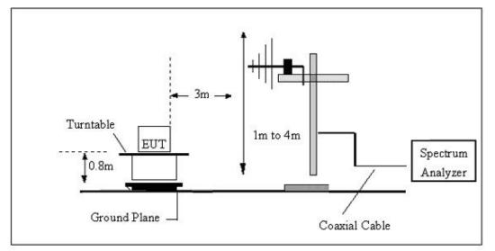
(C) Radiated Emission Test-Up Frequency Above 1GHz
