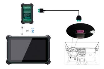
2)For the standard OBD II diagnostic socket, its connection as below:
