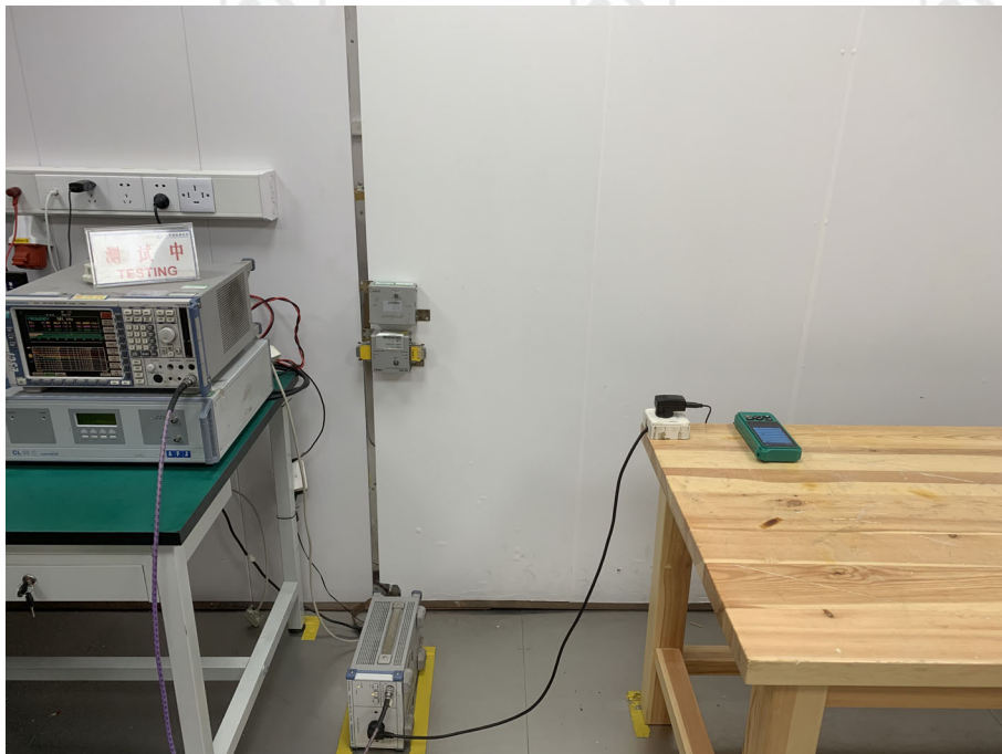
AC Power Line Conducted Emission
