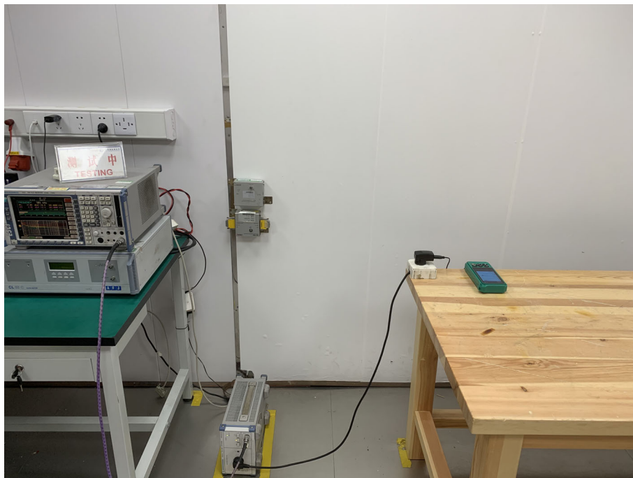
Conducted Emissions Test Setup
